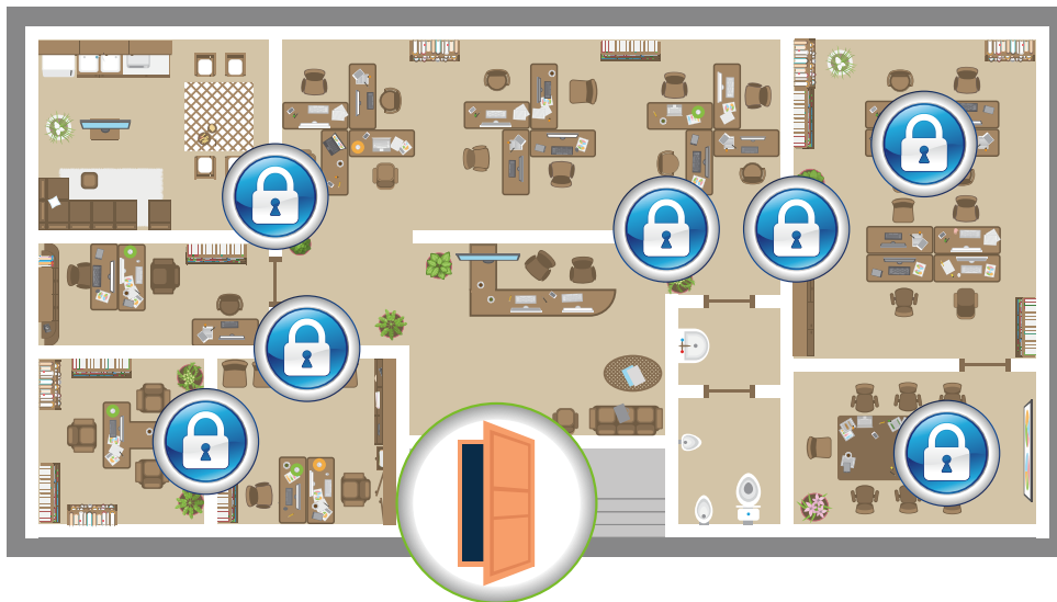
One door is open, at the same time, the others cannot open
