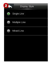
2. On the **Display Style** interface, you may select **Single Line**, **Multiple Line** or **Mixed Line** for the display of user information.
