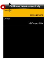
The Wiegand format and parsed card number are automatically detected.
