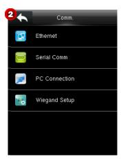
Set the parameters for the communication between the device and a PC, including the IP address, gateway, subnet mask, baud rate, device number, and connection password.
