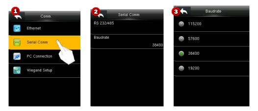
When the device communicates with a PC in serial mode, check the following settings.
