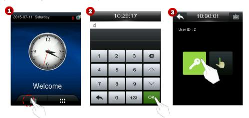
4. On the displayed interface, enter a password, and click **OK**. If the verification succeeds, the device plays the voice prompt "Thank you." and "Successfully verified." is displayed on the screen. If the verification fails, the device plays the voice prompt "Wrong password." and "Failed to verify." is displayed on the screen.
