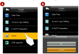
Note: After reset, the user information in the device and the settings on the access control interface are not deleted.
