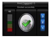
Enrollment succeeds. If the enrollment fails, the system will display a prompt message and return to the [Enroll Fingerprint] interface. In this case, you need to repeat the operations of step 2.
