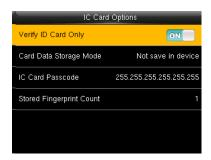
Verify ID Card Only: If this parameter is set to "YES", you pass the verification only after card verification. If this parameter is set to "NO", you need to verify your password or fingerprint after card verification.
