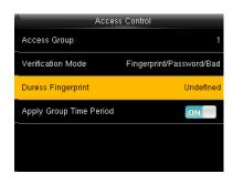
Press ▼ to select Duress Fingerprint and press OK.
