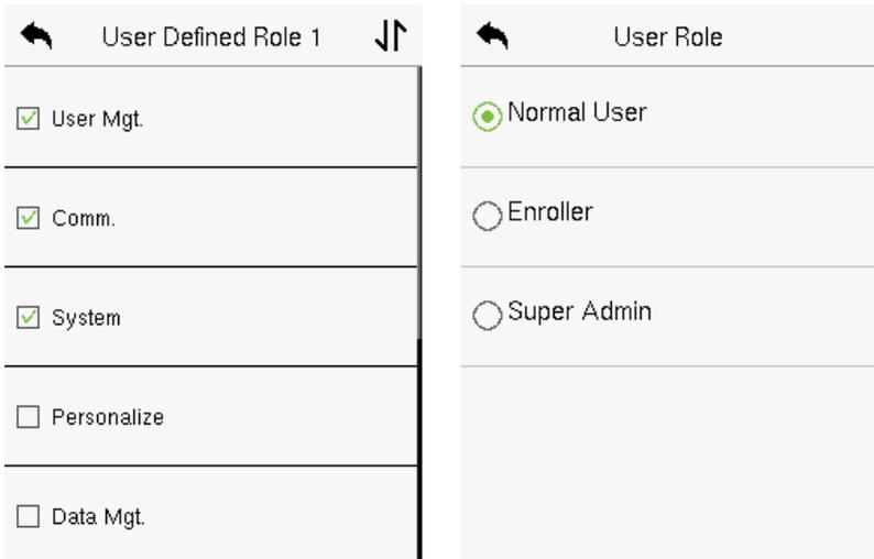
**Note:** If the User Role is enabled for the Device, tap on **User Mgt. > New User > User Role** to assign the created roles to the required users. But if there is no super administrator registered in the Device, then the device will prompt "**Please enroll super admin first!**" when enabling the User Role function.
