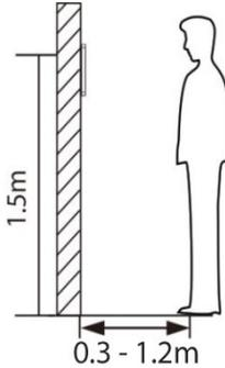
The distance between the device and a user whose height is in a range of 1.55m to 1.85m is recommended to be 0.3 to 1.2m. Users may slightly move forward or backward to improve the character of facial images captured.
