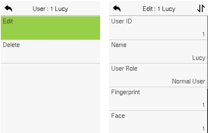
**Note:** The process of editing the user information is the same as adding a new user, except that the User ID cannot be modified while editing a user. The process in detail refers to "6.1 User Registration".
