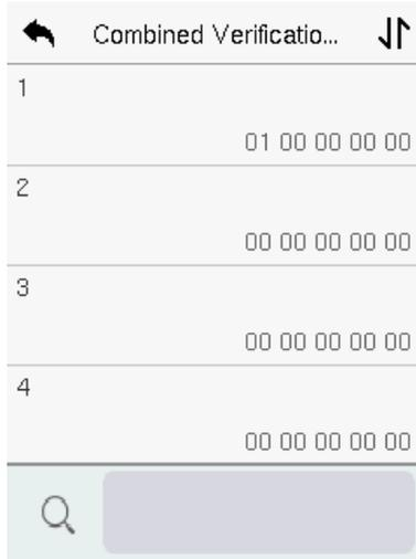
On the combined verification interface, tap the Door-unlock combination to be set, and tap the **up** and **down** arrows to input the combination number, and then press **OK**.
