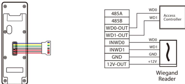
**Note:** 485A and 485B can be connected to the Barrier gate or the 485 Reader, separately, but cannot be connected to the gate and reader at the same time.
