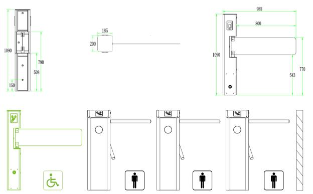
SBT1000S is usually used with other types of turnstiles together. It is suitable for trolleys, wheelchair passthrough, and is not suitable for high-traffic volume.
