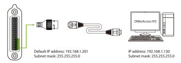
Click [COMM.] > [Ethernet] > [IP Address], input the IP address and click [OK]. Note: In LAN, IP addresses of the server (PC) and the device must be in the same network segment when connecting to ZKBioAccess IVS software.
