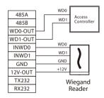
Note: 485A and 485B can be connected to the Barrier gate or the 485 Reader, separately, but cannot be connected to the gate and reader at the same time.
