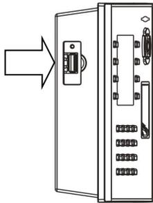
Insert U disk into USB slot of fingerprint sensor through mini USB cable.
