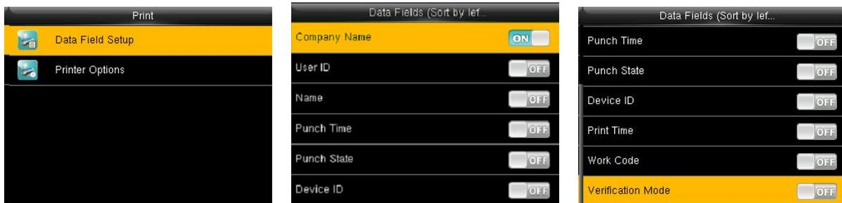
Press **▶** to select Data Field Setup and press OK.
