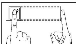
2) Improper finger placement: Not flat to the surface, off-centre, slanting.
