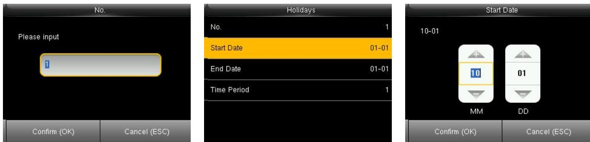
Enter the No. using keypad. Press OK.
