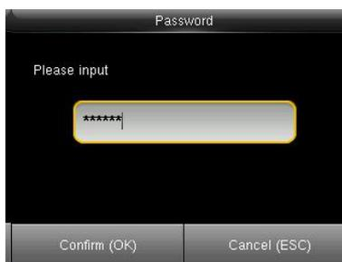
Enter a password using keypad then press OK..The FFR terminal supports the 1- to 8-digit passwords by default.
