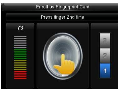
Place the same finger on the fingerprint collector for three consecutive times correctly. For details, see [1.1 Finger Placement](#)
