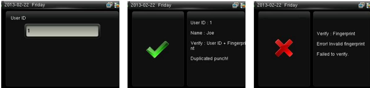
Enter the user ID using keypad on the initial interface. Then press OK. Place the enrolled finger properly on the fingerprint sensor.
