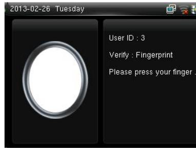
Place the enrolled finger properly on the fingerprint sensor.
