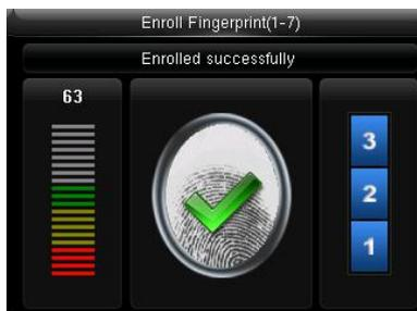
Enrollment succeeds. If the enrollment fails, the system will display a prompt message and return to the [Enroll Fingerprint] interface. In this case, you need to repeat the operations of step 2.
