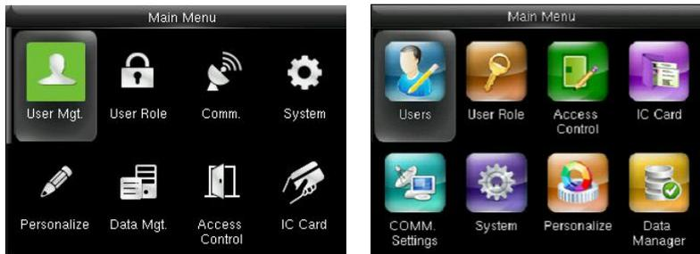
When the device is on initial interface, press M/OK to open main menu, as shown below:
