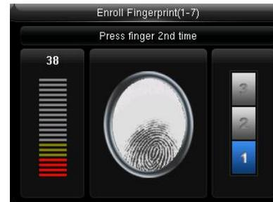
Place the same finger on the fingerprint sensor for three times.
