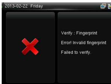
When verification failed, an interface shown above.
