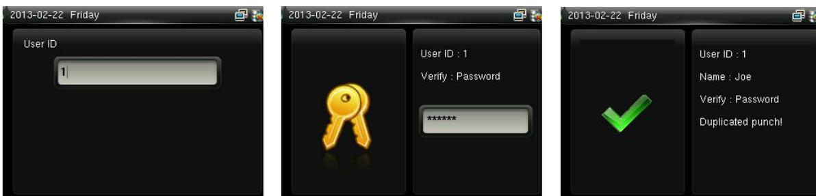
Enter the user ID using keypad on the initial interface. Then press OK.
